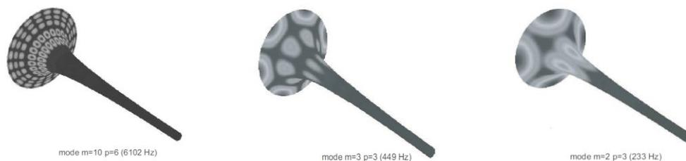
These pictures indicate that the structure is diametric and that it runs the length of the body of the instrument.
