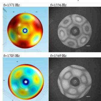
Figure 2: Elliptical modes of the vibration of the trumpet bell, as calculated from a 3D simulation (left) and observed using electronic speckle pattern interferometry (right).
